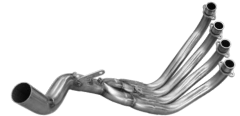
Honda CBR650, CB650, CB650F Stainless Steel Pipe With Slip-on Weight 4.975 kg
